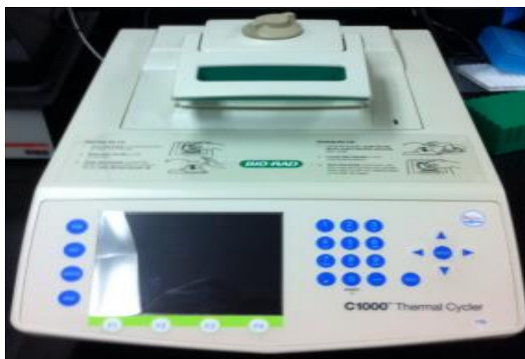
Figure 7. The thermal cycler is used to carry out PCR reaction. Image by Walter Suza.
